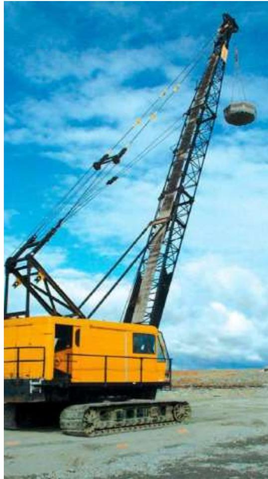
*(Fig. No.12) Demonstrates the equipment used in the Dynamic consolidation method*
